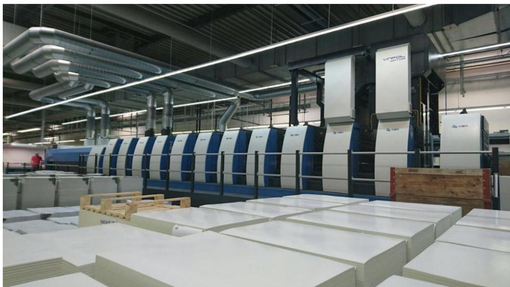
The Vinfoil Optima installed at SCHELLING AG on their new KBA Rapida 106
